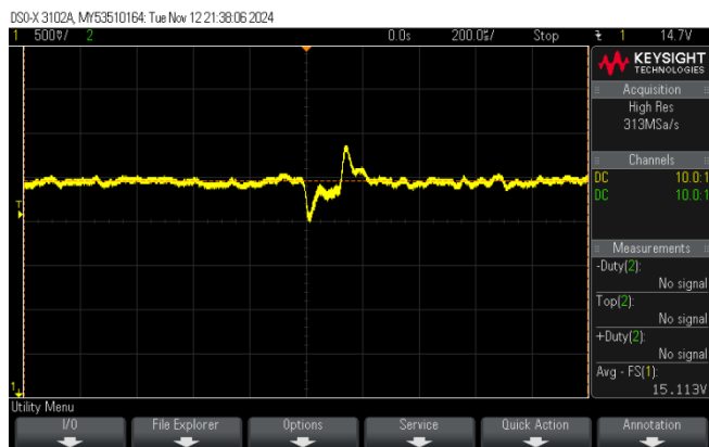
Figure 3 :Transient Response (VIN=28V, IOUT= 5-10A, 0.1A/us, No external COUT)
