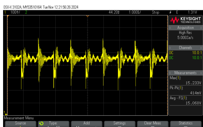
Figure 6 :Output ripple (VIN=28V, IOUT=10A, CR, No external COUT)
